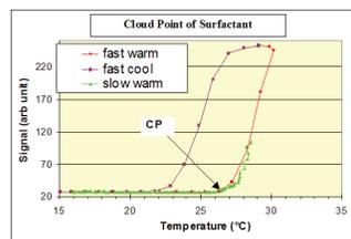
70Xi screen displays real-time test results and phase plot, showing temperature change and signal strength as test progresses. The graphic visual information helps users better understand anomalous behavior.
