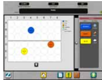
70Xi screen displays fully programmable 48-position vial selection and positioning. Samples are identified by ID number and color-coded by type. User selects sequence on-screen; no need to physically touch samples.
